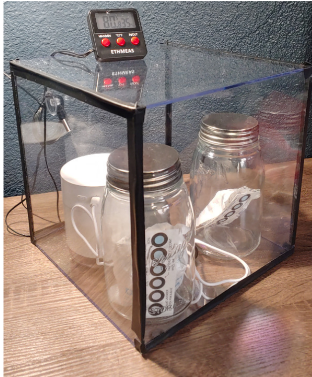
Figure 6. Photo of the Acrylic Plexiglass humidity chamber with humidifier unit, hygrometer and containment units (mason jars) to hold the desiccants
